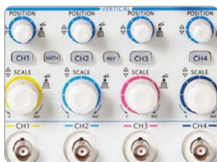
Independent Channel Control 4 analog channels with independent vertical control
